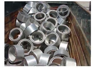
Figure 21.2 shows the segregation into a roll-off of Category Two filter elements, (filters cases and the HEPA filters).
